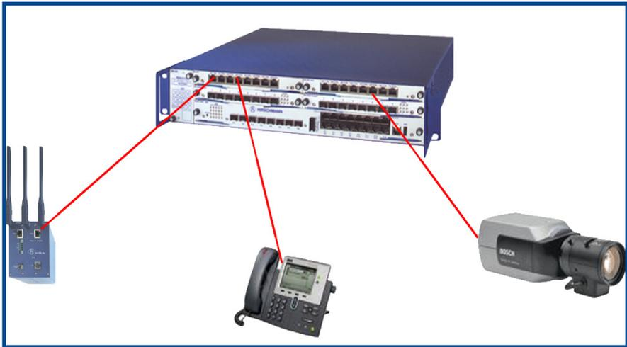
Figure 2.7: PoE endspan power insertion
