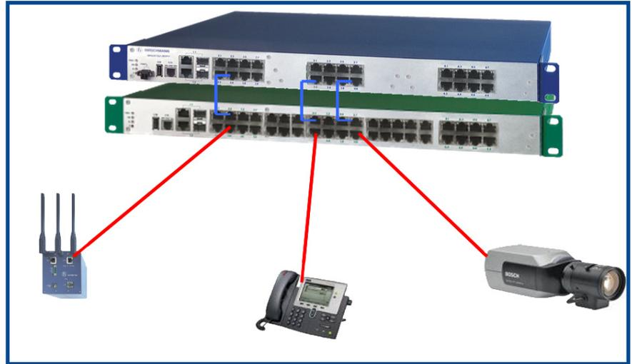
Figure 2.6: PoE midspan power insertion
